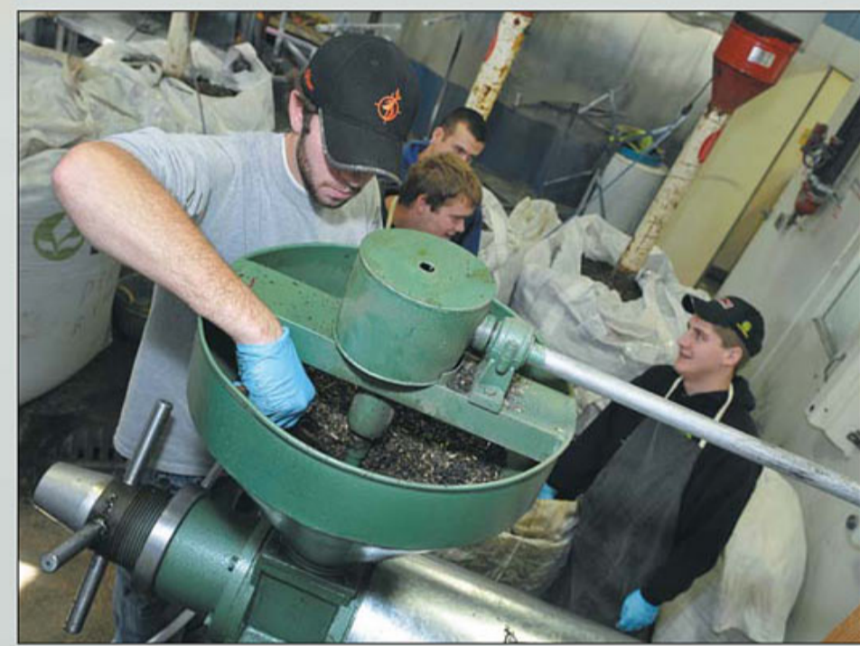
Isaac Hartung worked to ensure the seeds moved through the press. Agriscience technology instructor Dwight Swenson said next year the press and biodiesel processor will be moved to a more permanent spot on campus and automated with augers.
