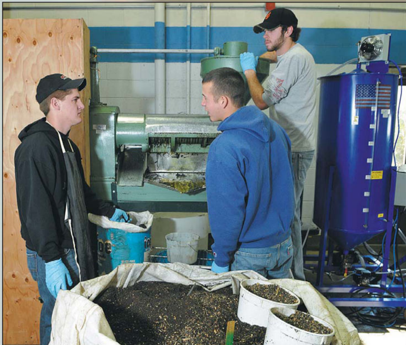
Agriscience students at Chippewa Valley Technical College used a seed press last week to press the oil out of canola and sunflower seeds. The students are, from left, Tom Seidl of Ogema, Mark Poeschel of Durand and Isaac Hartung of Elmwood. The biodiesel processor on the right will be used next month to turn the seed oil into biodiesel.
